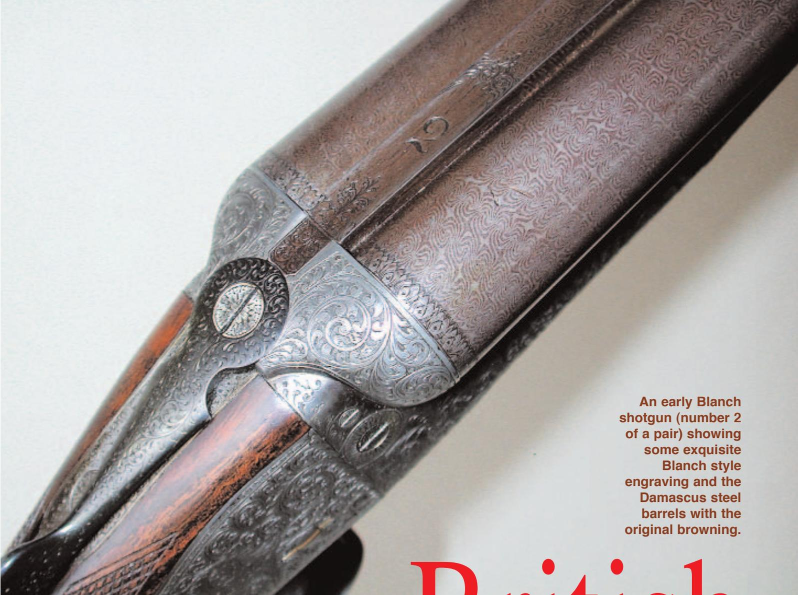
An early Blanch shotgun (number 2 of a pair) showing some exquisite Blanch style engraving and the Damascus steel barrels with the original browning.
